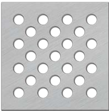
Round perforations from .016" (0.4 mm) hole diameter in stainless steel with .016" (0.4 mm) plate thickness; from .008" (0.2 mm) hole diameter in stainless steel plate up to .008" (0.2 mm).
