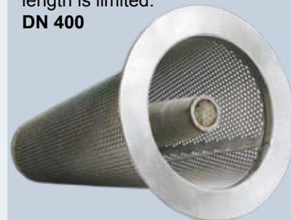
Protective strainers are applied in the pipeline construction in front of pumps, compressors or control valves. Depending on the process, particles will be filtered out from water, condensate or gas, in order to protect the plant components from damage.
