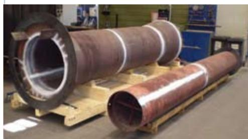
Strainer made of 16 Mo 3 drilled DN 600
